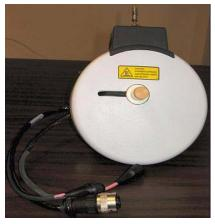
Figure 15 Multimode Spray Chamber
